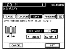
Utilizing this feature allows the facing pages of a book or magazine to be copied page by page onto two separate sheets of paper or duplex-copied on one sheet. There is no need to move the original on the glass. You can also place a pair of A4 (B5 or LT) sized originals side by side and copy them on separate sheets of paper.
